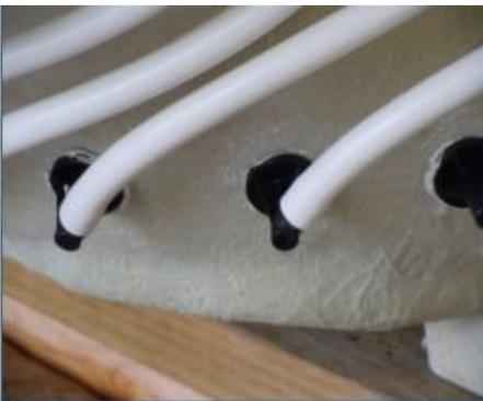
Real jets drain water into the tub naturally. The design is key to a clean air system. All the air supply lines are attached above the jets, so gravity removes most of the water. Then auto purge dries the air supply lines.
